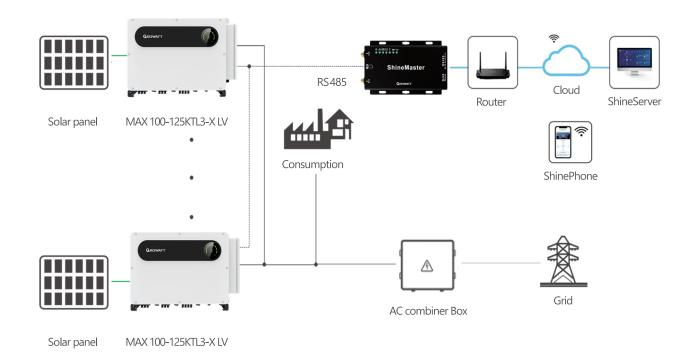
Growatt provides system solutions of monitoring and smart energy management for C&I projects, ShineMaster is a monitoring device for multiple inverters in one system, and SEM provides the solution for special system functions, such as system export limitation or system PF control.
