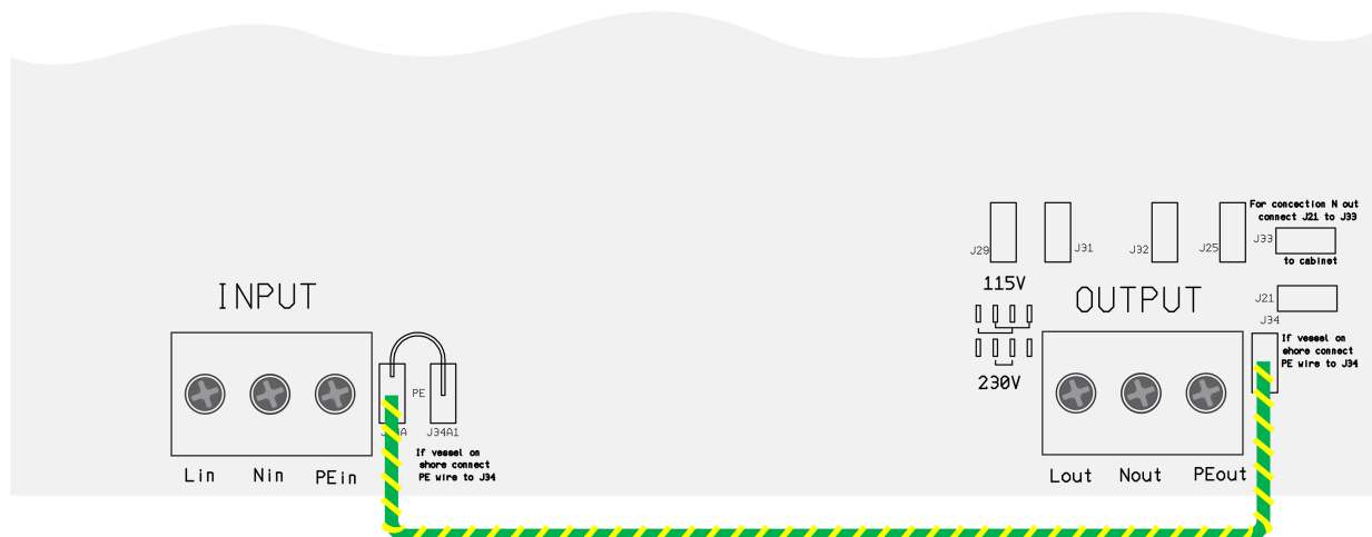
AC input earth is connected to AC output earth when the vessel is out of the water (on land) during winter or for maintenance.
